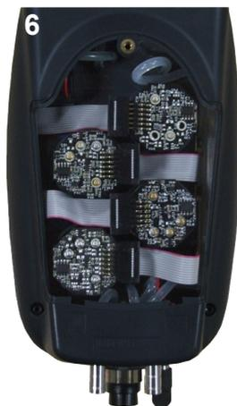
Connection of the sensor ribbon cable
