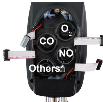
\* NO<sub>2</sub>, SO<sub>2</sub> and CH<sub>4</sub> sensors
